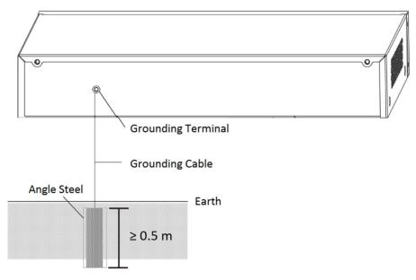
Figure 3-2 Grounding with Angle Steel
