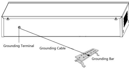
Figure 3-1 Grounding with Grounding Bar
