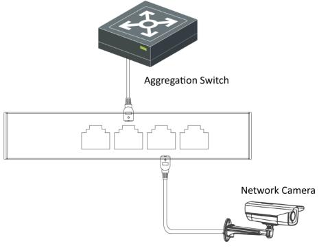
Figure 3-3 RJ45 Port Connection
