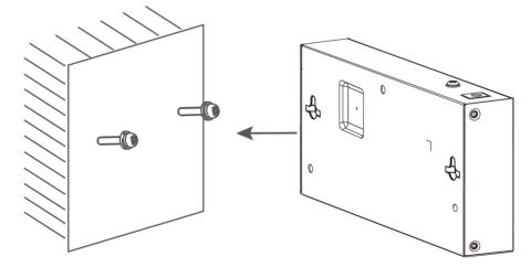
Figure 2-1 Wall-Mounted Installation
