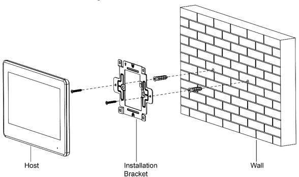
Figure 2-1 Surface installation
