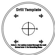
Figure 2-12 Drill Template of the Junction Box
